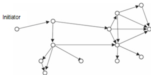
Figure 6. The flood mechanism.
